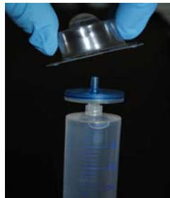
Attach filter to syringe, twist until 'tight', about 1/2 turn, remove filter cover and discard
